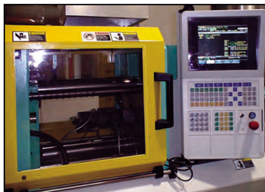
MPL recommends injection molding rheometry to generate optimum data for Moldflow simulations.
