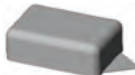
Model with the part and fan gate designed in the CAD system
