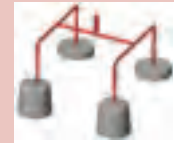
Family mold with a hot runner system
