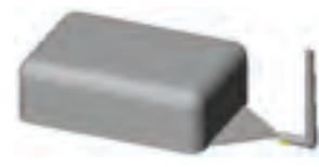
Sprue and runner added to the fan gate model to complete the runner system
